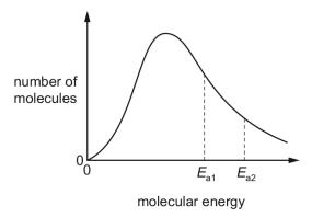
$E_{\rm a}$  is used to represent the activation energy for the reaction between the gases. Of the two values shown, one is the activation energy for a catalysed reaction, the other for an uncatalysed reaction.
